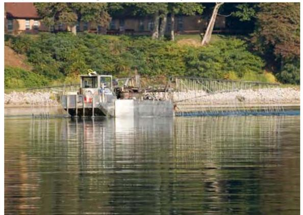
**Figure 19.** Alum application barge.
